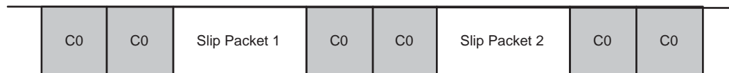
Figure 3.1: SLIP Packets with 0xC0 at the Start and End of Each Packet
