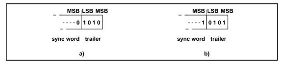
Figure 6.7: Trailer in CAC when MSB of sync word is 0 (a), and when MSB of sync word is 1 (b).
