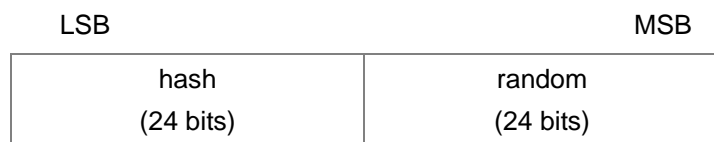
Figure 1.3: Format of random device address
