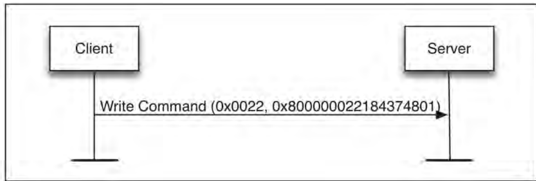
Figure 4.13: Signed Write Without Response example
