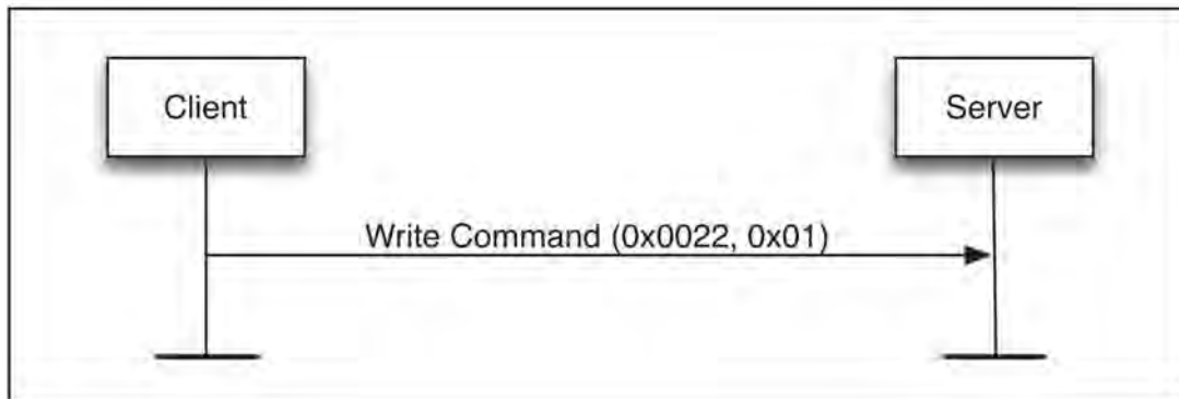
Figure 4.12: Write Without Response example
