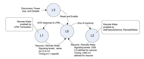
Figure 1-1. LPM State Transition Diagram
